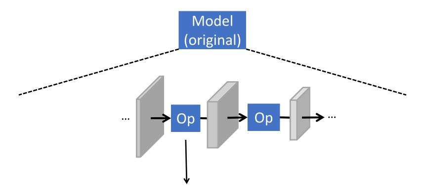
• Example operators: convolution, max pooling, ReLU, ...
